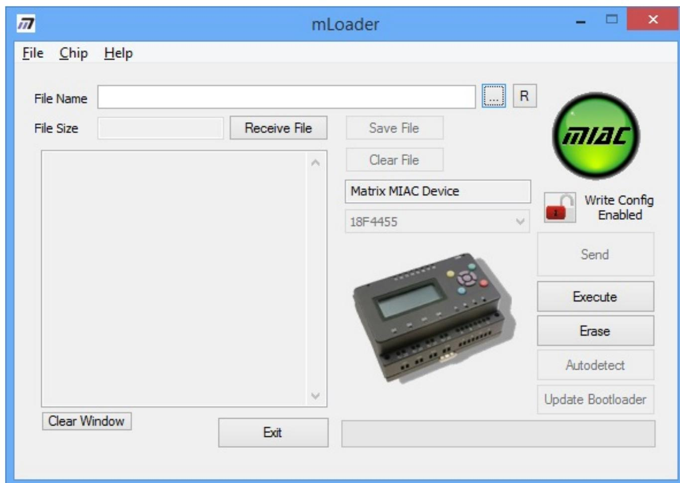
If mloader did not detect the MIAC we need to put it in bootloader mode by **pressing the RESET button**, this should hopefully get your MIAC into the state
