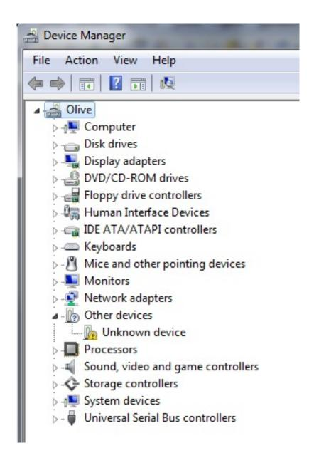
Make sure this is your Matrix device by unplugging the device and the yellow exclamation mark should disappear. When you plug it back in it should re-appear.
