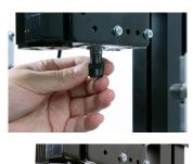
Place the collet into the motor assembly and secur in place using the collet holder; do not tighten
