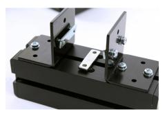
Slide the Tool Post & Motor Assembly onto the Short machine bed ensuring the three clamping plates locate into the T-slots of the Tool Post.
