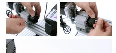
To secure a workpiece into the 4 Jaw Chuck use the 2mm Allen key to adjust the position of each Jaw individually, there are guide lines on the face of the chuck to help centralise the workpiece.
