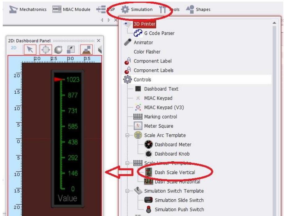
Set the scale component properties, such as the minimum, maximum and resolution values.
