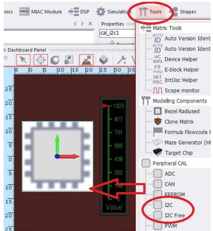
Set the I<sup>2</sup>C properties, such as the Baud Rate, to match the device.
