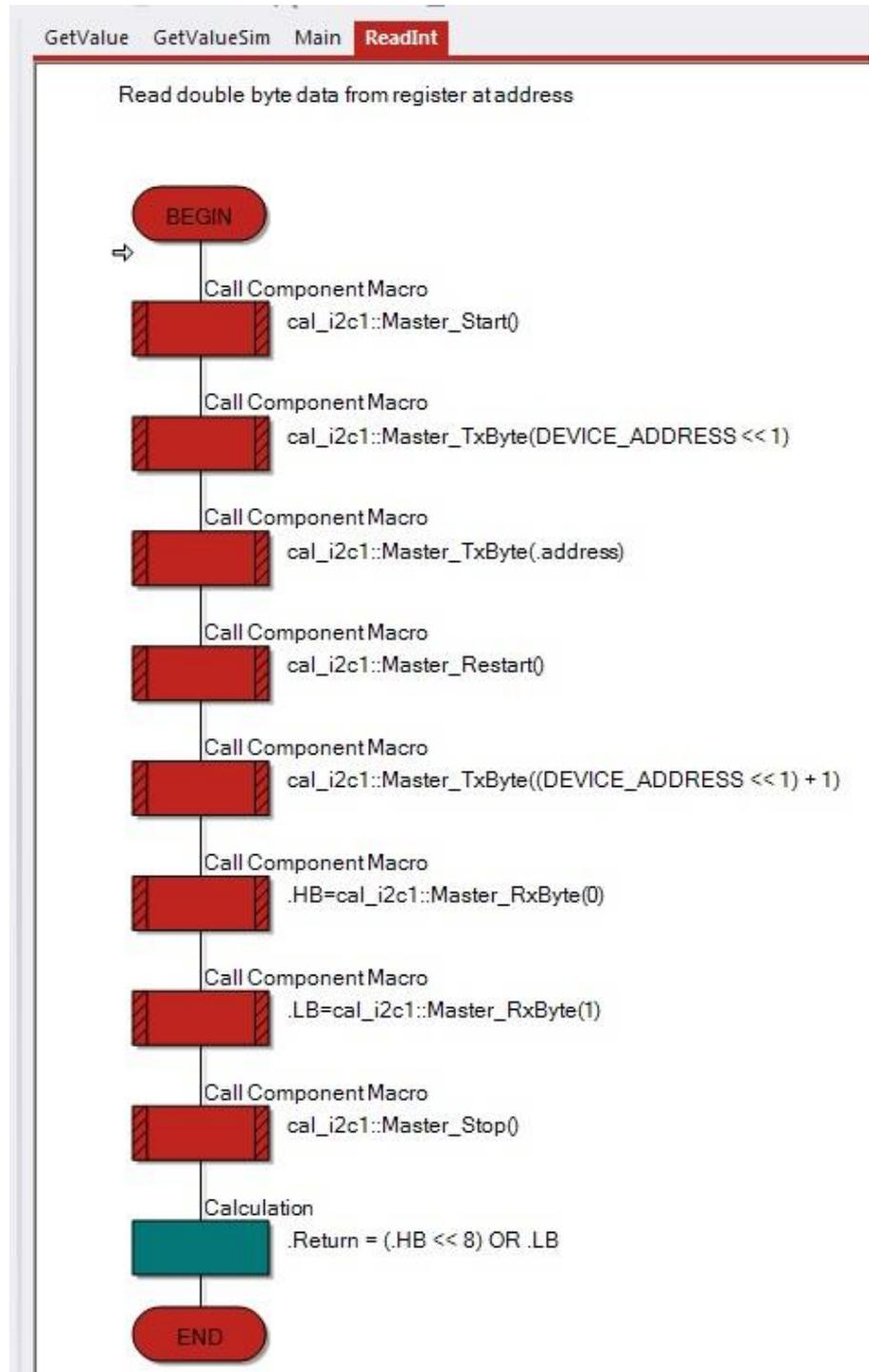
For this particular device the digital temperature is read from the first two locations of its internal registers.
