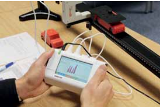
The datalogger included is fully self-contained and has a VGA output for connection to a projector for class demonstrations.
