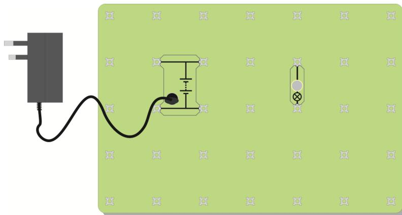
You have just used two circuit symbols, one standing for a battery, or group of batteries, and the other for a lamp, or sometimes any kind of indicator.
