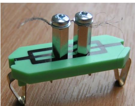
Tease out one or two strands of wire wool from the pack. Carefully clamp them across the gap of the sampler, as shown in the photograph.
