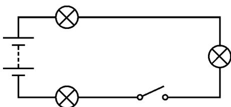
Here is the same circuit, drawn using symbols, Compare the two versions of the same circuit diagram!
