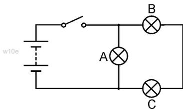
The 'blobs' above and below bulb A mark junctions in the circuit.
