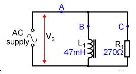
Remove the connecting link at **A**, and connect a multimeter, set to read up to 20mA AC, in its place. Record the current flowing at point **A** in the table. Remove the multimeter and replace link **A**.
