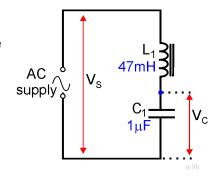
Change the frequency to 200Hz, repeat the measurements and record them. Do the same for the other frequencies listed, and complete the table.
