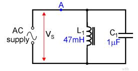
Remove the connecting link at **A**, and connect a multimeter, set to read up to 20mA AC, in its place. Record the current flowing at point **A** in the table. Remove the multimeter and
