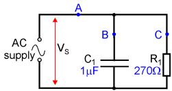
Remove the connecting link at **A**, and connect a multimeter, set to read up to 20mA AC, in its place. Record the current flowing at point **A** in the table. Remove the multimeter and replace link **A**.
