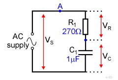
Remove the connecting link at **A**, and connect a multimeter, set to read up to 20mA AC, in its place. Record the current flowing at point **A** in the table.
