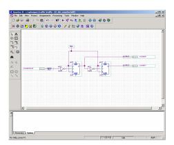
Quartus II design software allows rapid development of CPLDs in block diagram, VHDL or Verilog format.
