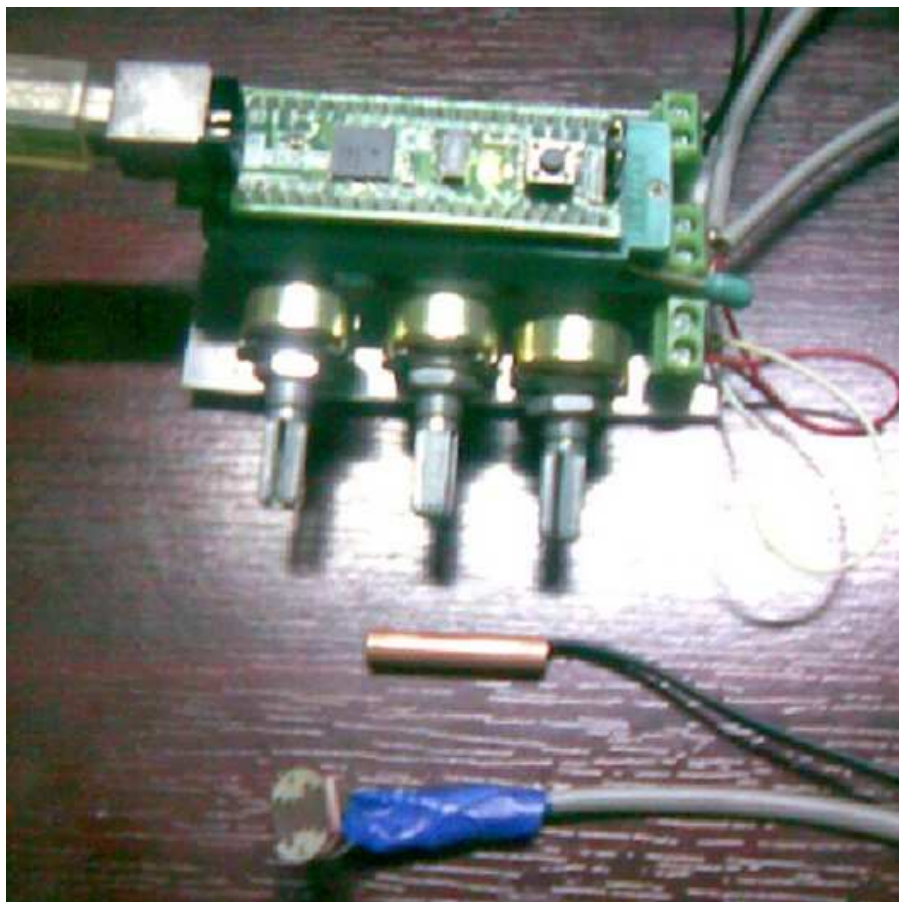
The picture above shows the ECIO as used in the NASOCT sensors hardware.
