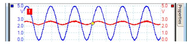
9 Move the Gain potentiometer fully clockwise, the output signal should now go from 0V to 5V in an almost square wave. The Clip LED should appear to be constantly on.
