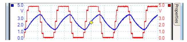
14 Keeping the gain set fully clockwise, adjust the filter pot so that it is fully anti-clockwise.
