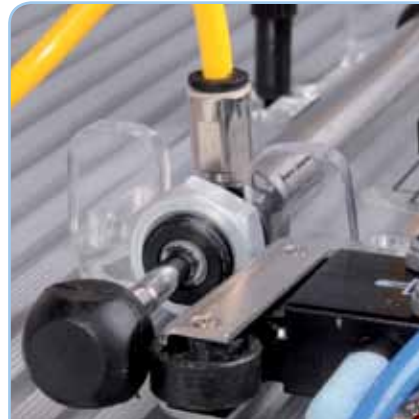
All pneumatic fittings are quick release
