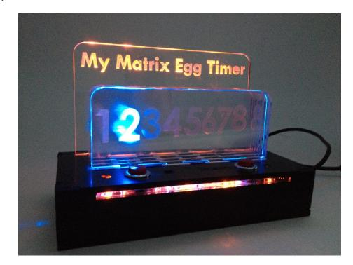
By using an engraving technique on the clear Perspex the bring LED lights up each number in turn. Here we have used 8 planes of Perspex with a small air gap between each panel to avoid light leakage across multiple numbers.
