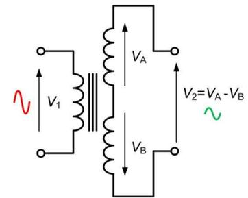
The LVDT requires an AC input, of a few volts amplitude with a frequency usually of a few kilohertz. This generates an alternating magnetic field, which is intensified in the core. This, in turn, induces an alternating voltage in the secondary coils. The greater the overlap of the core and the secondary coil, the greater the voltage induced.
