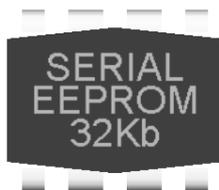
The dsPIC and ATmega MIAC versions have an internal Serial EEPROM (non-volatile memory) device for which the component can be added to a project to give read and write access.
