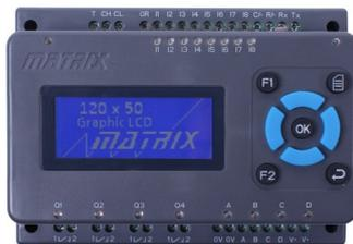
To deploy your project to the AVR (Arduino-Compatible) versions of MIAC, connect via a USB cable and apply power to the MIAC.
