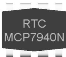
The dsPIC and ATmega MIAC versions contain a Real Time Clock that has backup power to keep the clock active for up to a few days without power.
