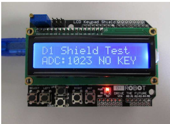
Arduino UNO with the D1 Robot shield fitted.
