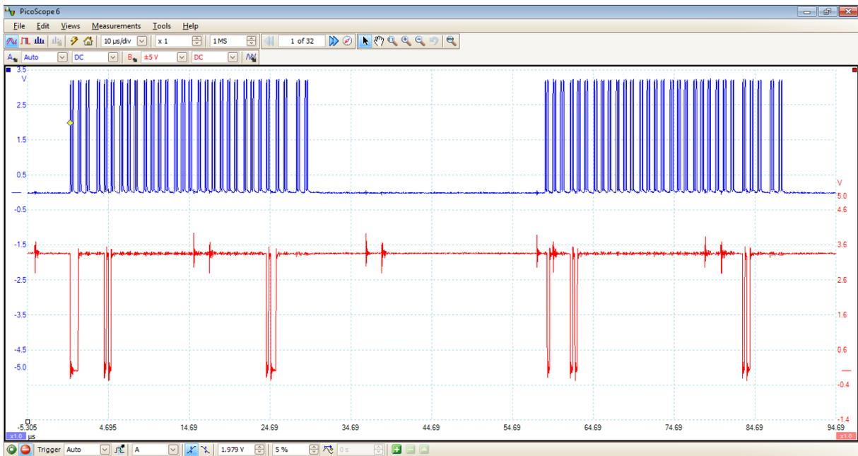
60 data clocks in blue are 28us long to make one line, with pause of 31us before next line starts. (I.e. is like a very long flyback on a CRT.) Data in red is one bit of a 4-bit bus. 59us per line x 240 lines = 14ms per frame = 71Hz refresh rate.
