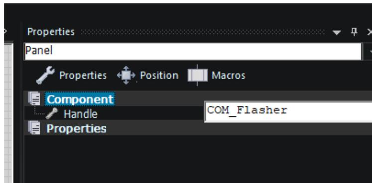
In order to get our automatic flashing arrows to work i.e. **once** during data transfer of - *outgoing data and incoming data respectfully*. To set this time delay for the **ON to OFF period**, we need an adjustable variable for controlling the flash time period. We can achieve this with a delay macro that uses a variable the user can change from the properties panel, **see** below.
