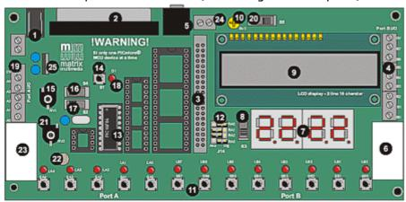
To set the PICmicro development board to the external analogue sensor mode set jumper 3 on the Port A mode selector J14.
