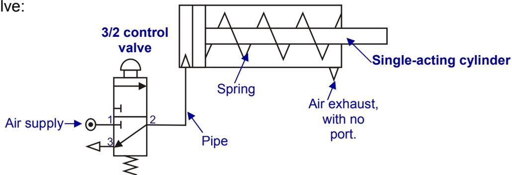
The control valve is described as a **3/2** valve because it has **3** ports and **2** states.
