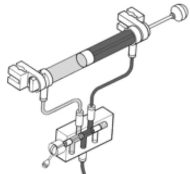
When the valve spring pushes the spool back, air flows from the manifold into the front of the cylinder to retract it. Air behind the piston can exhaust through port 5.
