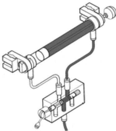
In the first diagram, the spool allows air to flow from the manifold into the front of the cylinder which keeps it retracted.
