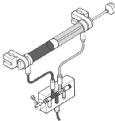
Here, air flows from the manifold into the cylinder to extend it. Air in front of the piston can exhaust through port 3.
