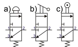
9. Which of the following is operated by a lever switch?
