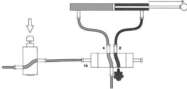
The spool inside the valve is moved from one position to another by compressed air. This is called a pilot/pilot five port valve. It has two extra ports, one at either end, called pilot ports and numbered 12 and 14. When air is sent to pilot port 14, the spool is moved to the position shown.
