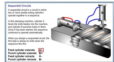
Animated example of a sequential circuit (in this case) used in a pneumatic stamping systems.
