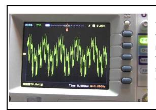
When the sample rate is much lower than the signal frequency, the resulting reconstruction is not a good representation of the original. It may even generate false output frequencies, known as aliases. Nyquist's sampling theorem specifies the minimum sample rate for a given signal.
