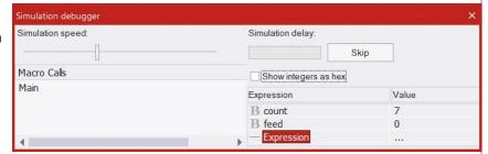
If you simulate a flowchart and then press the pause button, you can click on variables in this window to change their value. This allows you to test your flowchart under known conditions.
