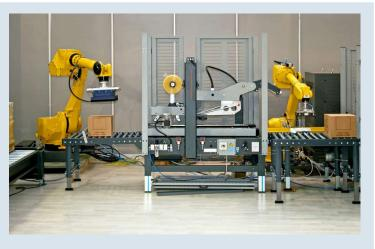
Photograph shows two robots in a packaging work cell.
