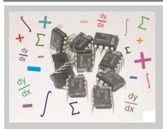
Operational amplifiers (op-amps) are everywhere. They are the most commonly used analogue IC, used in audio systems and instrumentation systems, used to perform mathematical operations, (hence their name,) such as addition, subtraction, and integral and differential calculus.
