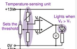
Near the switching threshold, any electrical noise could push the signal over the threshold, and cause the output to switch rapidly on and off, from the noise alone. If this is the case, it may be better to use a Schmitt trigger circuit.
