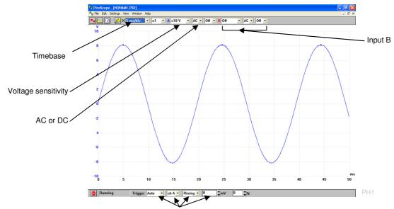
Trigger—when / how the trace starts
