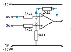
Earlier we pointed out that the ideal op-amp has infinite input impedance, and so draws no current from its input source. We will assume that this op-amp is ideal!
