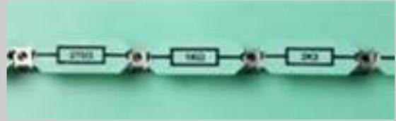
In a series connected circuit there are no alternative routes and no junctions for the current. The same current flows through each of the series-connected resistors.
