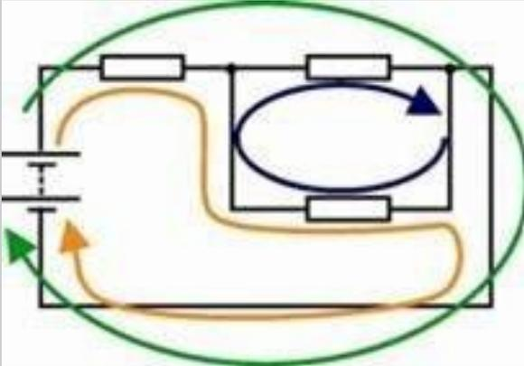
Around any loop in the circuit, the algebraic sum of voltages is zero.
