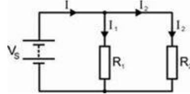
The current  $I$  from the power supply splits into  $I_1$  and  $I_2$  at the junction.
