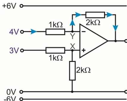
Earlier we pointed out that the ideal op-amp has infinite input impedance, and so draws no current from its input source. We will assume that the op-amp used here is ideal!
