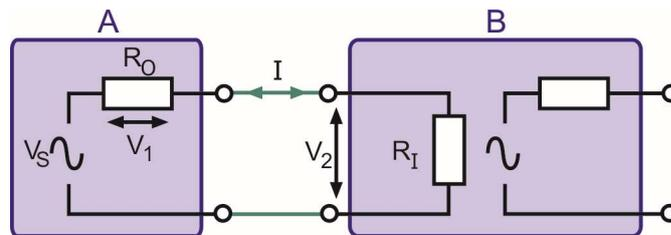
The diagram shows two subsystems, **A** and **B**. Our design aim is to pass on as much of the voltage  $V_S$  as possible. In other words, we want  $V_2$ , the voltage 'seen' by **B**, to be as close as possible to  $V_S$ , the voltage generated by **A**.
