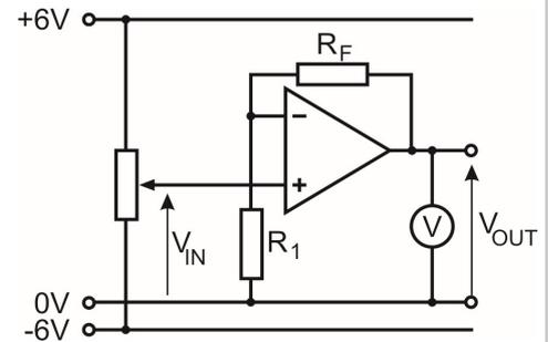
$R_F = 1\text{k}\Omega, R_1 = 1\text{k}\Omega$
