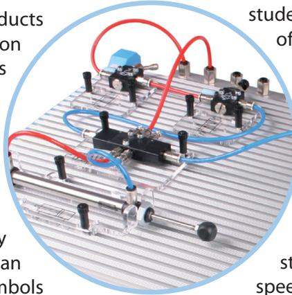
Automatics also integrates electrical components and even a USB programmable microcontroller, so that students will gain familiarity with the most modern of software controlled systems.
