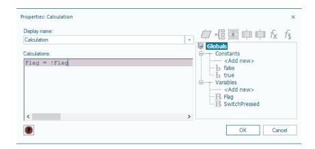
Our final command is to output the status of Flag to the LED. We do this with an output command, as we did in the first example. However, rather than writing a 1 or 0 in the 'Variable or Value' box we write the variable name Flag.
