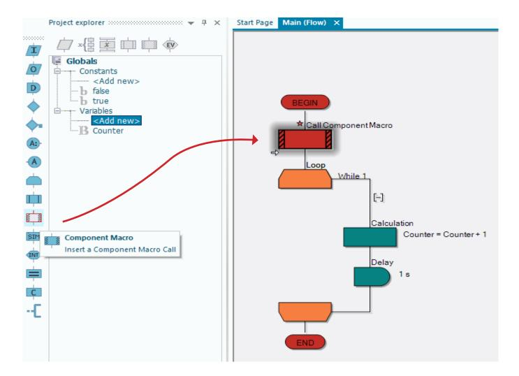
Open its configuration properties, as usual, by double clicking on the component macro. You will see the box below. Press the + button next to the LCD\_4x20 component to access the available component macros.
