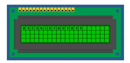
What we need to do is clear the LCD screen each time we write a new value. Luckily for us executing a clear screen routine also moves the cursor position back to (0,0). Add another component macro above the PrintNumber macro, and configure it to 'Clear'.
