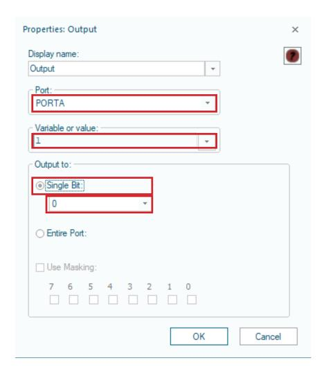
To make an LED flash we must turn it on and off. Place another output icon on your flowchart, below the original, and configure it as before. Although this time you should write a value of 'o' instead to turn our LED off.
