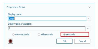
Currently we turn our LED on for 1 second, then we turn it off. However, we do not hold the LED off and so it will turn on again very fast. It would therefore appear that the LED is always on. We must add another delay icon after we turn the LED off, which can be seen in the final flowchart below.
