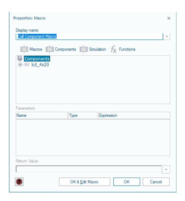
Once opened you will see a list of 13 component macros available for the LCD screen. These are all pre-written sub routines, developed by Matrix, to assist you with using the LCD screen. The first we want to use is 'Start'. Select Start and press 'OK'.
