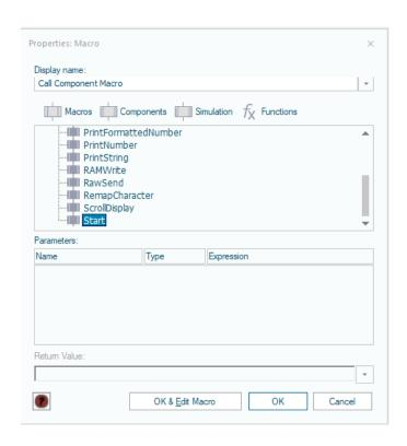
The Start routine is required to initialise the LCD screen, so that the microcontroller knows it exists, and sets up timing routines etc.
