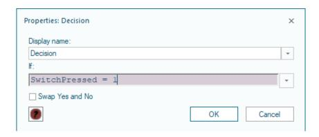
Since we are creating a latch we only want to modify the value of Flag when the switch has been pressed. Therefore, we will only place code in the 'Yes' branch of the decision. We leave the 'No' branch empty. Once the switch has been pressed we want to toggle the value of Flag from 0-1 or vice versa.
