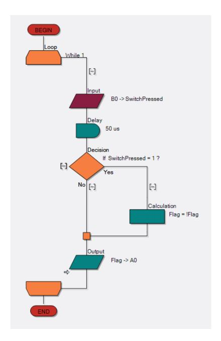
You should now both simulate and download your code to hardware for verification. As you press the switch on your board, the appropriate LED should illuminate, and stay that way until you press the switch again. Once confirmed working, move onto the final exercise.
