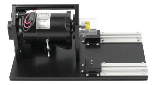
The aluminium cradle which houses our dynamometer features a rugged and safe sliding mechanism into which each of the other six motors in the range fix into position. The motor coupling meets the dynamometer in a protected housing and allows for safe study of each machine type at 24 volts. When using our system in manual mode, it is likely you will require two (per set) HP1324 Fluke 115 True RMS Digital Multimeter and one HP8067 Tektronix Digital oscilloscope.
