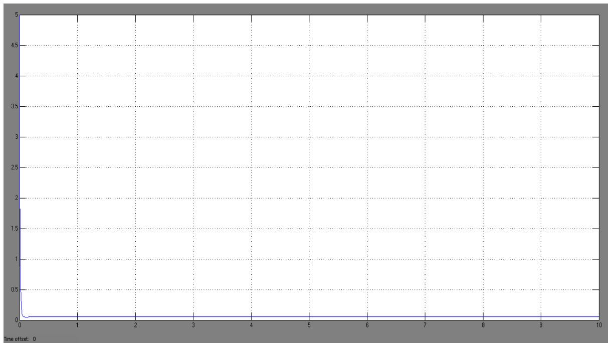
Figure 20: Error of the closed loop system with only P control, K_p=100
