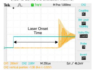
Examination of laser onset time delay as a function of different pump powers, levels of intra cavity loss and output coupling ratios.
