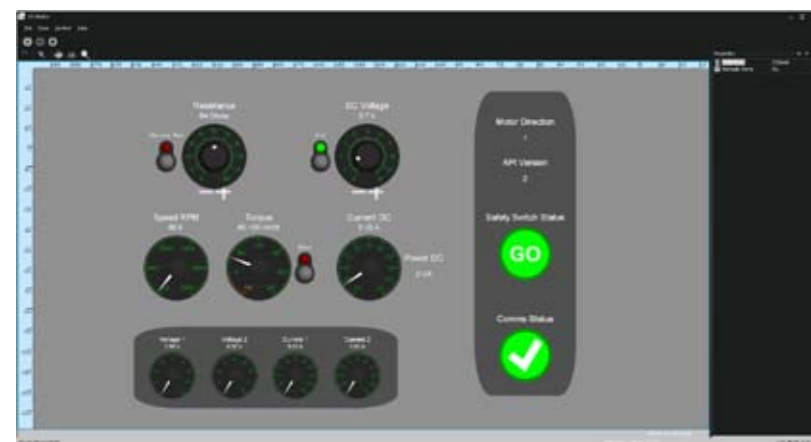
Above: The machines can be controlled manually, using the control box provided or through a PC based environment. Different panels are used, dependent on the motor type being studied.
