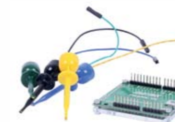
Stand-alone FlowKit 2 with USB lead and test clips The standard FlowKit is provided with 4 test clips.
