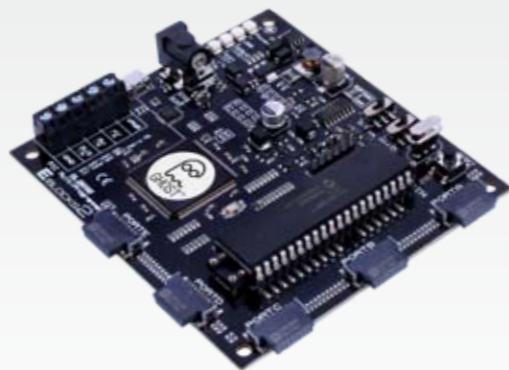
BL0080 PIC Multiprogrammer board
