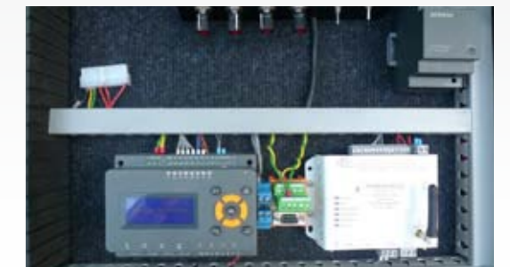
A dsPIC MIAC's CAN bus capabilities being used in an automotive application. Only the MIAC can handle CAN and Modbus without 'extra' extensions, it is easy to program, it has a build-in display and function keys
