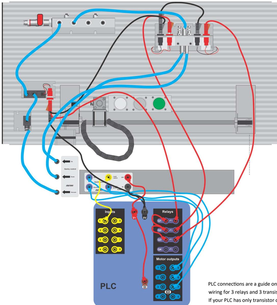
PLC connections are a guide only and show wiring for 3 relays and 3 transistor outputs. If your PLC has only transistor outputs then adjust accordingly.
