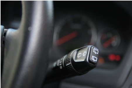
Indicator stalk houses several types of switch
