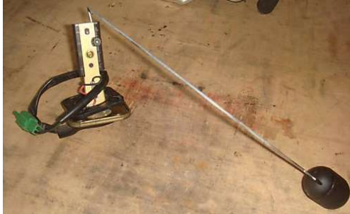
Fuel sensor with float
