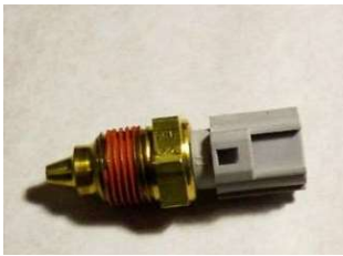
Coolant temperature sensor - single resistor type
