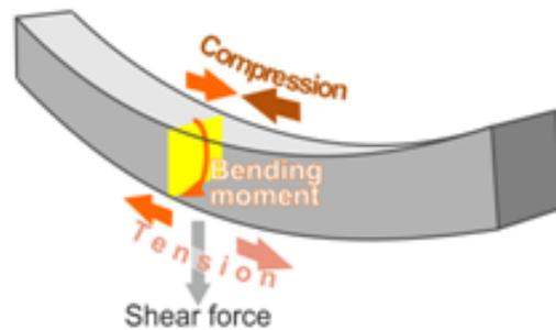
Internally, the attractive forces between these particles, viewed at a cross-section cut through it, can be considered as a combination of a resultant force and a resultant couple. This resultant internal couple is called the **bending moment**. The resultant internal force is called the **shear force**.
