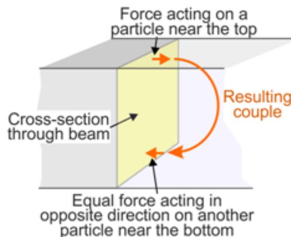
The second diagram illustrates the idea of a bending moment. Looking at a cross-section through the beam, the compressive force on a particle somewhere near the top is the same but opposite to the tensile force on a particle near the bottom. Together they form a couple trying to distort the beam. Adding together the effects of all such particles results in a bending moment.
