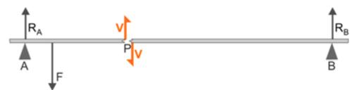
The equation given above shows that the force F is bigger than reaction  $R_A$ . Hence the shear force V must act vertically upwards to keep section AP in equilibrium.
