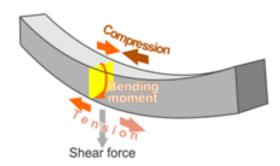
Internally, these forces, viewed at a cross-section cut through the beam, can be looked on as a combination of a resultant force and a resultant couple. The resultant internal couple is called the **bending moment**. The resultant internal force is called the **shear force**.
