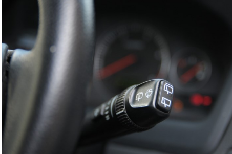
Indicator stalk houses several types of switch
