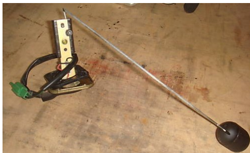
Fuel sensor with float
