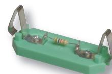
If the component on a carrier should become damaged then it is easy to replace with a soldering iron. Note that damage to potentiometers is very easy and because of this a high wattage, low value, resistor is added to the wiper of many potentiometers to limit current.
