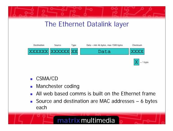
In the Datalink layer we can see the fundamental MAC packet structure.
