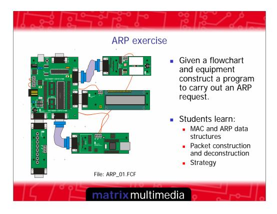
This is the layout of the equipment in the internet solution – there is a Multiprogrammer with a 16F877 PICmicro, a sensor board on port A, a LCD board on port B, the Internet board sites on port C, and a switch board on port D.
