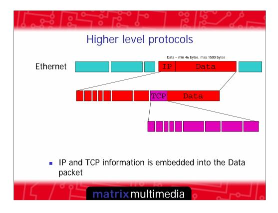
At higher layers in the OSI model the data packet is nibbled away by additional data at each layer. So IP data is embedded in the MAC data frame, and TCP data is embedded in the IP data frame.
