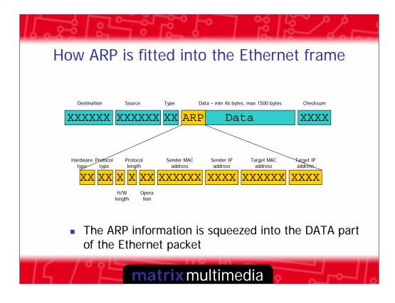
ARP simply take up 28 bytes of the Data section of the MAC layer to insert other relevant information about the ARP. ARP is used by computers to determine an IP address from a known MAC address.
