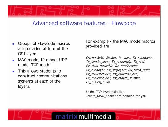
Flowcode and the internet solution are designed to provide a flexible learning platform that allows students data structures, communication flow in a digital system, and programming strategy. The families of macros at the MAC, IP, TCP, and UDP layers are a key, and unique, feature here. Flowcode allows students to build on their understanding at each level before they progress onto the next.
