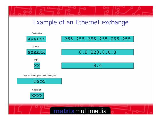
Looking in more detail at the Datalink layer: The Ethernet protocol is part of datalink and already we see the collection of numbers separated by full stops which is familiar to anyone who has set up an internet connection.
