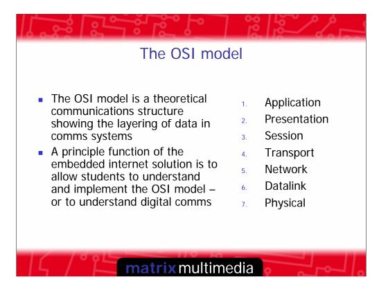
The OSi model is a theoretical model that demonstrates the information layering process in digital communications systems. At the lowest level we have the types of wires used, the voltage levels etc. The 0's and 1's of the physical layer are grouped into packets with error correction in the Datalink layer and further information is added into the packets at each subsequent layer- including application specific data at the top layer.
