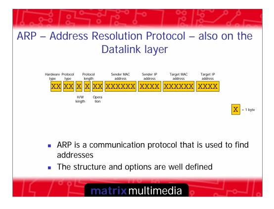
Address Resolution Protocol – or ARP – is also in the Datalink layer. It has a slightly different packet structure and this is built on the MAC layer as you will see on the next slide.
