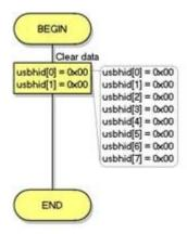
The clear data array software macro simply assigns 0 to all eight of the outgoing data bytes. This is the equivalent of no keys being pressed.
