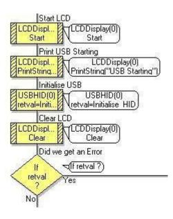
The program starts by initialising the USB component and waiting for the USB device to be recognised by the computer. The return value from the initialise function is used to determine if we have a successful connection or not.
