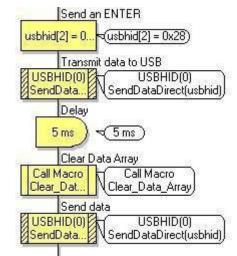
The end of the program loop assigns an enter to the outgoing data buffer to allow the numeric data to be saved into the cell in Excel and move onto the next cell.
