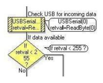
The program checks for incoming data by calling the ReadByte hardware macro. If the return value is less then 255 then we have valid data, otherwise no data has been received.
