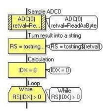
If we are sampling then sample the voltage connected to the ADC pin specified by the ADC component and then convert the numeric value into a string of characters. For example the number 255 would be converted into the characters '2', '5' and '5'. The program then enters a loop where each character in the string is converted into a key press and sent on to the computer. After each key press is sent the outgoing buffer is cleared and resent to represent a key release.
