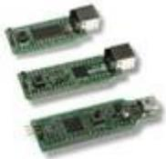
ECIO devices are powerful USB programmable microcontrollers with either 28 or 40 pin standard DIL (0.6") footprints. They are perfect for student use at home, project work and building fully integrated embedded systems.
