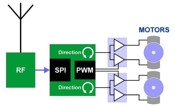
The two ADC channel readings sent by the transmitter are used to independently control the speed and direction of the two motors, allowing skid steering of the chassis.
