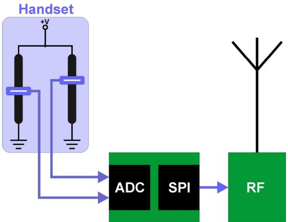
The first two bytes of the transmitted message contain the sampled values from the ADC channels connected to the handset potentiometers (the other two bytes are for future expansion).
