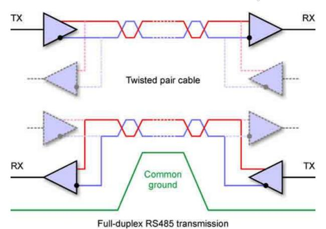
This configuration can be used as a direct replacement for a standard RS232 connection, allowing greater distances and higher Baud rates. It can also be used as the master node in a simple network..
