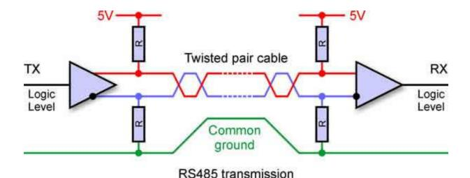
RS485 is often used for serial data communications. The lack of a specific protocol means that several pre-existing ones have been adopted (with some adaptations to allow additional benefits of RS485 to be included), and new ones developed for specific applications.
