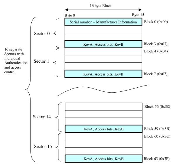
1024 byte memory is organised as sixteen sectors, each of which is made up of four blocks and each block is 16 bytes long. The first block in the memory (Block 0) is read-only and is set in the factory to contain the four-byte serial number (UID), check bytes and manufacturers data.
