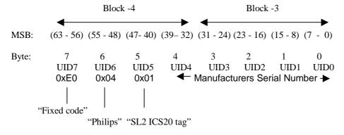
ISO15693 defines that UID0 - UID5 (bits 0-47) contain the manufacturer serial number. (UID4 and UID5 can contain information on capacitor value, IC and customer identification).
