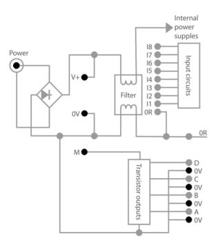
The MI0235 8 bit PIC MIAC transistor outputs are not powered internally. The M terminal is used to apply power to the transistors which allows a voltage other than the supply voltage to be used on the transistor outputs.
