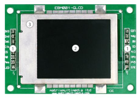
Mirrored SIL Pin Connections 2.54mm Pitch
