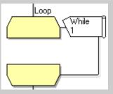
The 'loop' function appears in all the worksheets. It makes the program cycle through repeatedly.
