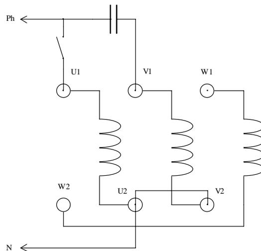
Two coils are set out of phase using a capacitor.
