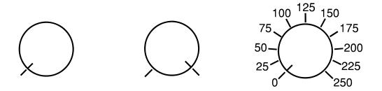
Divide the distance rotated between the two pencil marks into equal divisions and draw a scale as shown in the right and diagram. Any small errors you may make will easily be absorbed by components tolerances.
