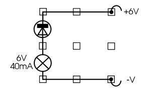
Turn on the supply to the circuit, then reverse the diode.
