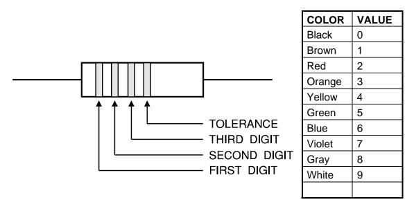
For example, a resistor with the following colored bands: brown, gray, brown, and gold would have a value of  $180\Omega$ , and a tolerance of 5%. Check under the  $180\Omega$  resistor carrier in the kit to verify this.
