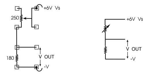
Now change the circuit to the one shown. This is an even simpler potential divider circuit.
