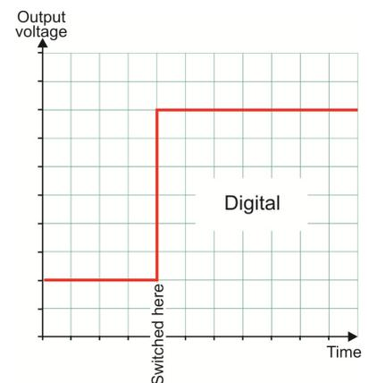
The vocabulary of digital electronics talks about these two voltages as 'logic 0' and 'logic 1'. Somewhere in a particular design, these will be defined, usually as a range of possible voltages. For example, logic 0 may be defined as any value between 0V and 1.0V, while logic 1 is any value between 10.0V and 12.0V. Giving a range of values recognises that signals can change a little as they move through an electronic system.
