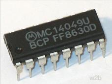
Logic gates can be built in a number of ways, which has led to a number of logic 'families' each with its own set of capabilities and limitations. One of these is called **CMOS**. The photograph shows a CMOS
