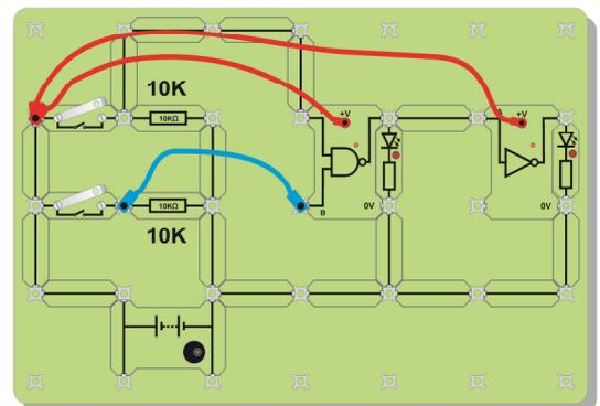
The NAND function can be generated by an AND gate followed by a NOT gate. Verify this by building and testing the circuit shown.
